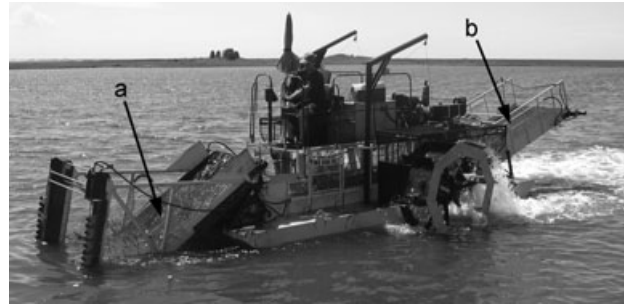
Figure 1. Commercial SAV harvester contracted in 2004. Zostera marina shoots are cut and collected on a conveyor belt (arrow a) for offloading to a separate transport boat (arrow b).
